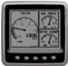
CANTrac 2600 Fully Programmable Graphic Display
